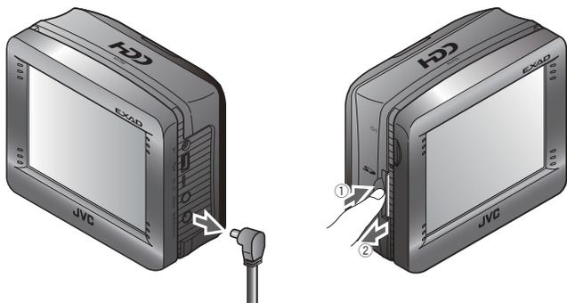
6. Slide the battery switch to “ON.”
