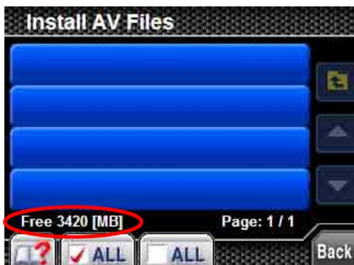
If the free space is smaller than 2 GB, delete files installed on the "Delete files" menu until the free space becomes larger than 2 GB.
